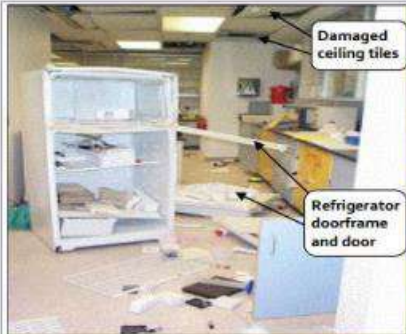
University of Vermont, June 2000: Flammable liquids stored in a refrigerator resulted in an explosion. The door blew off and debris propelled across the room.
